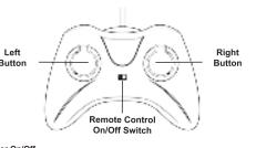
Power On/Off Slide the ON/OFF Switch to ON to turn on the Remote Control. Slide the ON/OFF Switch to OFF to turn off the Remote Control.
