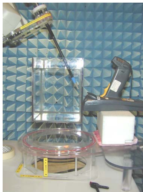
Figure 35. Positional photograph of PDT687C in the End on, separation 0.0mm.
