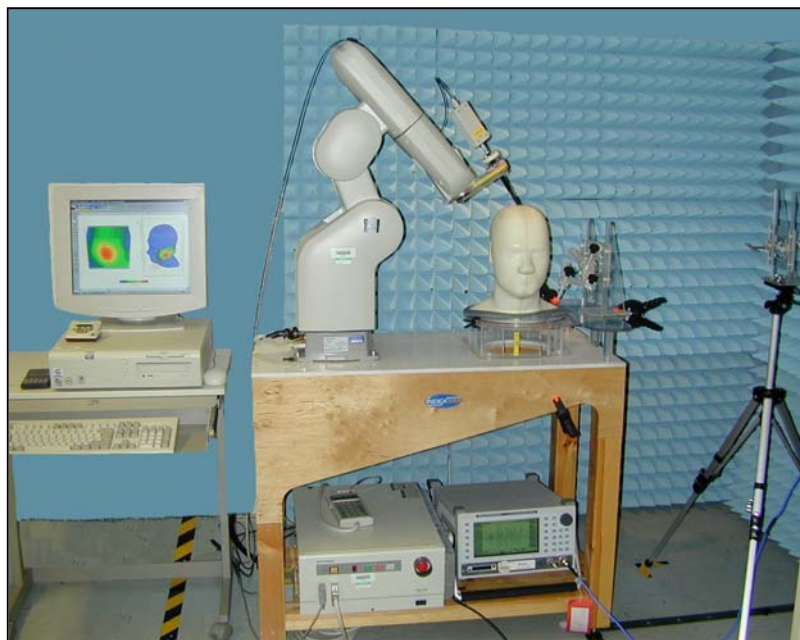
Figure 13: Principal components of the SAR measurement test bench
