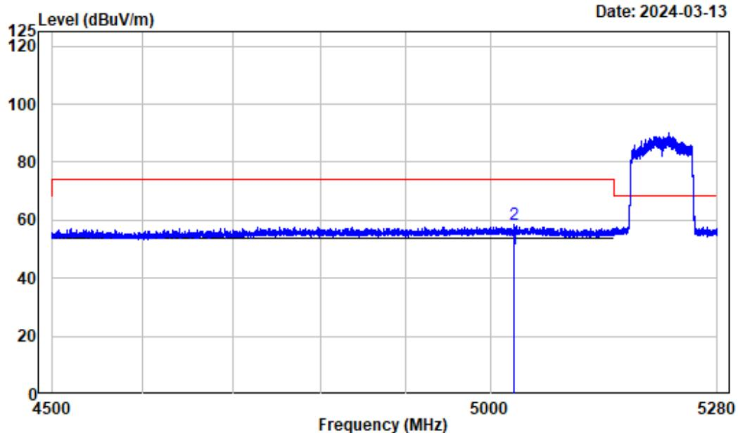
**802.11ac80**Test Channel: **5210MHz** Ant. Polar. : **Horizontal**
