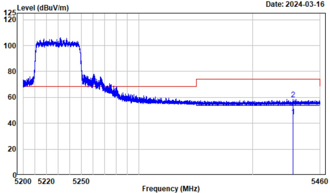
**802.11ax40**Test Channel: **5230MHz** Ant. Polar. : **Vertical**
