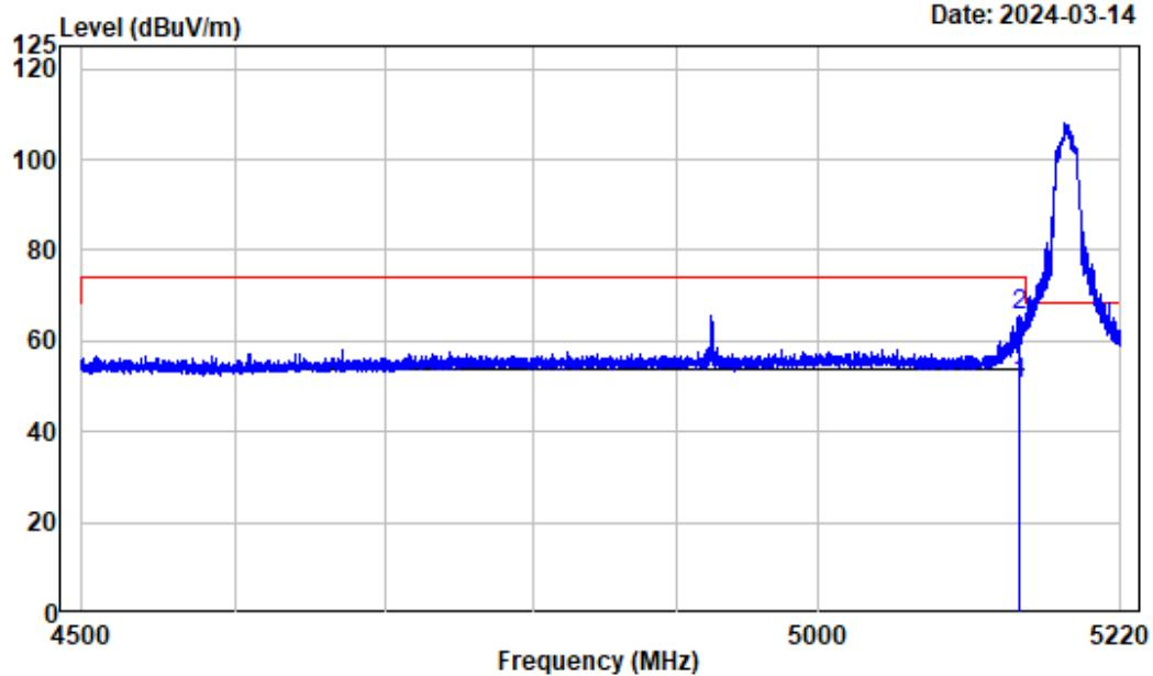
**802.11a ANT 1**Test Channel: **5240MHz** Ant. Polar. : **Horizontal**
