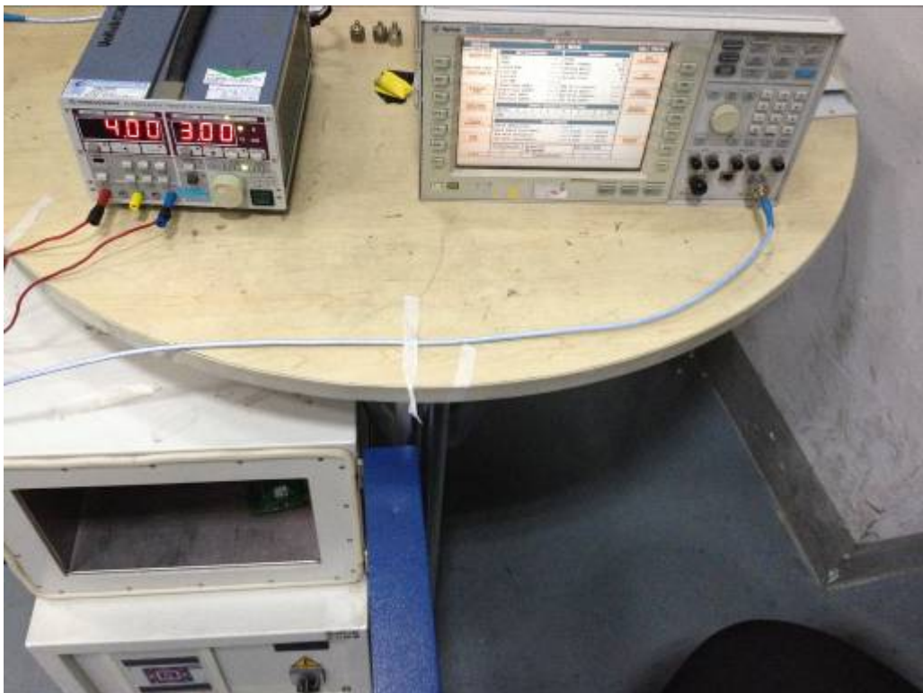
Frequency Stability Under Temperature & Voltage Variations Setup
