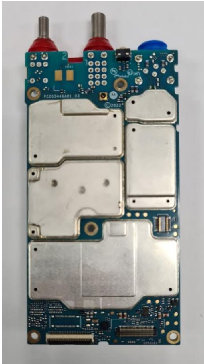
RF board with Shields (Top) of TIA NKP Model
