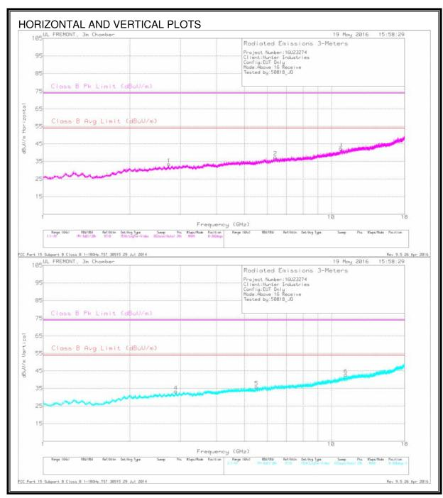
For measurements above 1 GHz the resolution bandwidth is set to 1 MHz, then the video bandwidth is set to 3 MHz for peak and average measurements.
