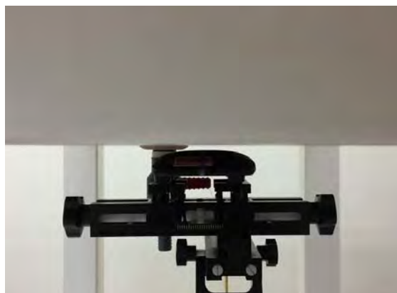
Fig.5 EUT Back side to flat phantom
