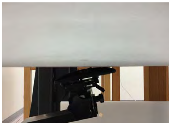
Fig.4 EUT Curve side to flat phantom
