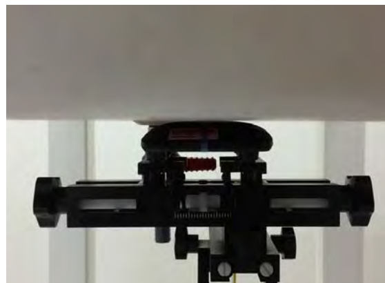
Fig.3 EUT Back side to flat phantom
