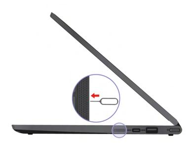
Step 2. Insert the SIM card in the SIM card tray. Note the orientation of the card and ensure that it is seated correctly.
