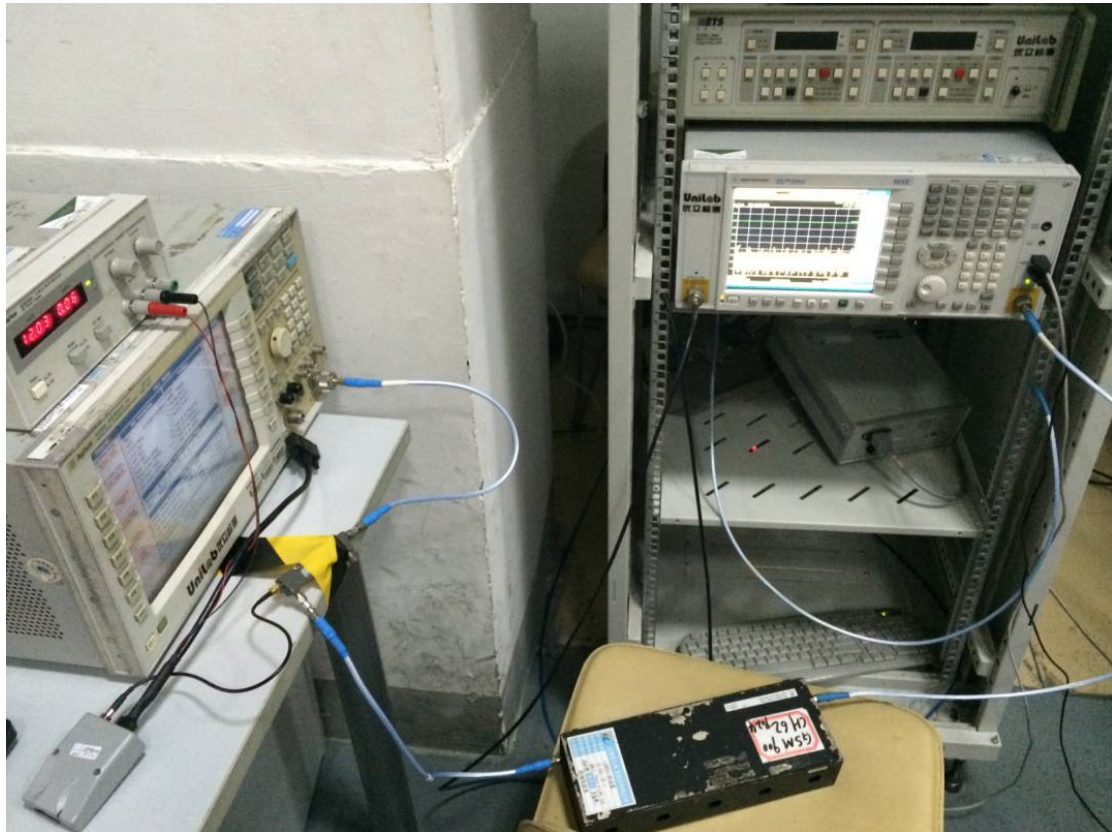
Frequency Stability Under Temperature & Voltage Variations Setup
