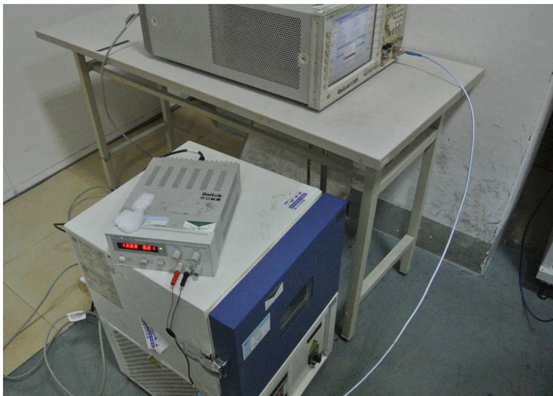
Frequency Stability Under Temperature & Voltage Variations Setup
