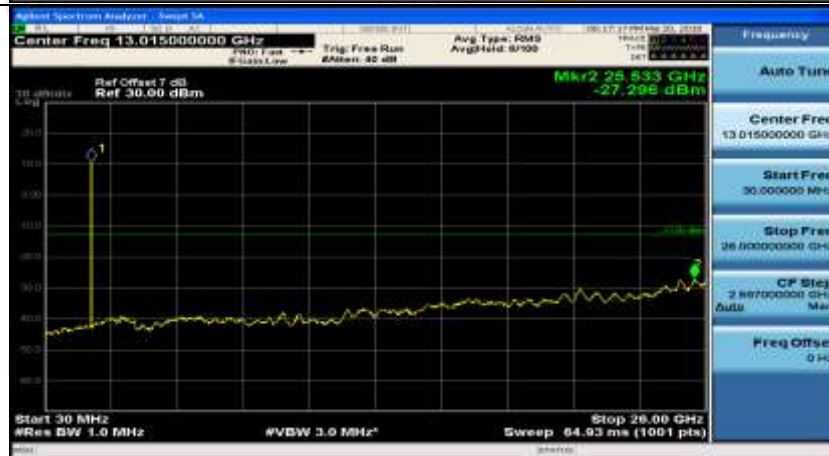
(Channel Bandwidth: 3 MHz)_MCH_16QAM_1RB#7
