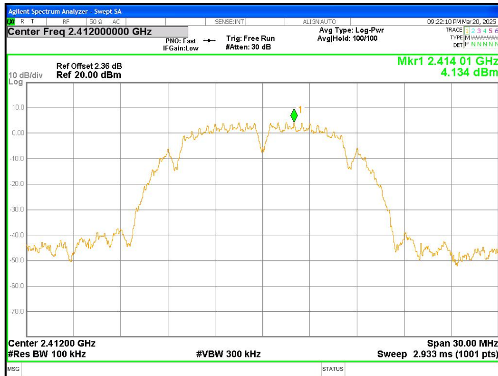
Band Edge NVNT b 2412MHz Ant1 Emission
