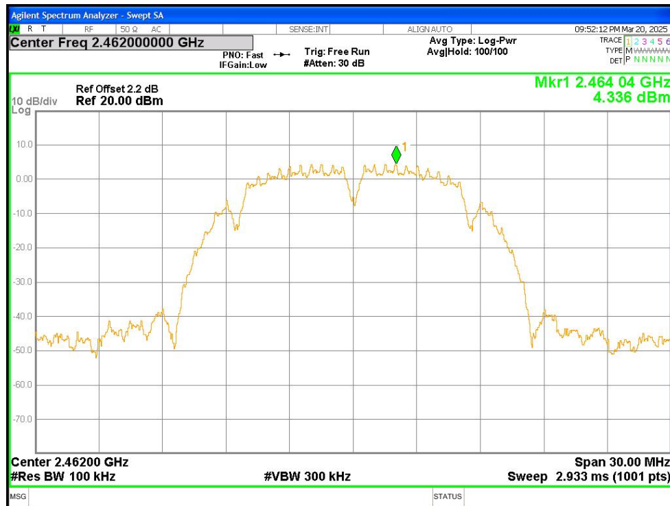
Band Edge NVNT b 2462MHz Ant1 Emission
