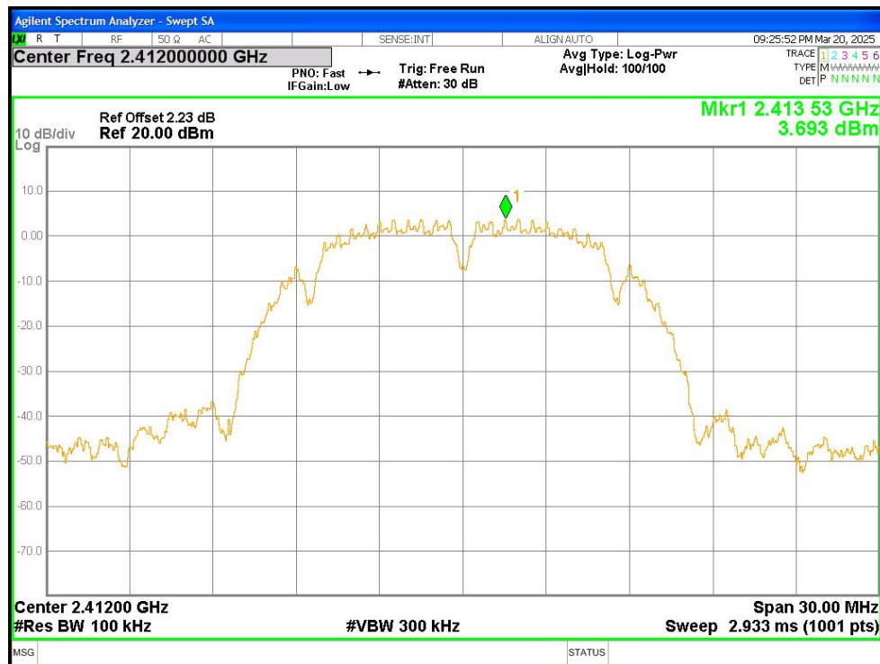
Band Edge NVNT b 2412MHz Ant2 Emission
