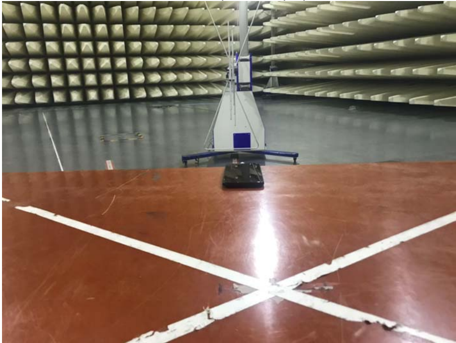
Radiated Emissions Test Setup (with charger) (30-1000MHz)
