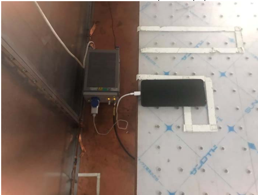
Conducted Emissions Test Setup (with charger)
