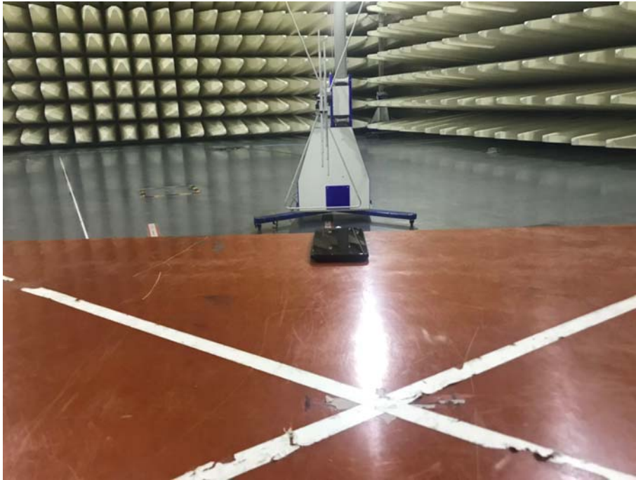
Radiated Emissions Test Setup(below 1GHz)
