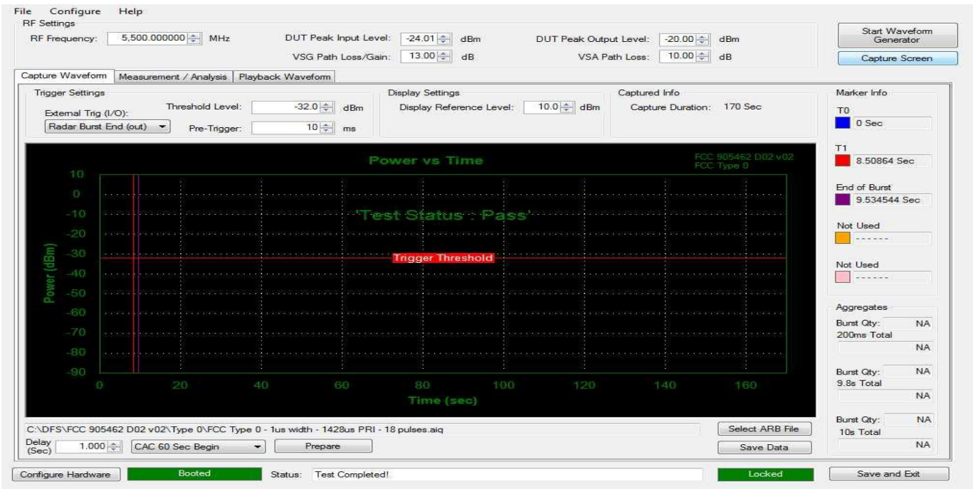
Figure 8.8-1: Radar burst at the beginning of the CAC
