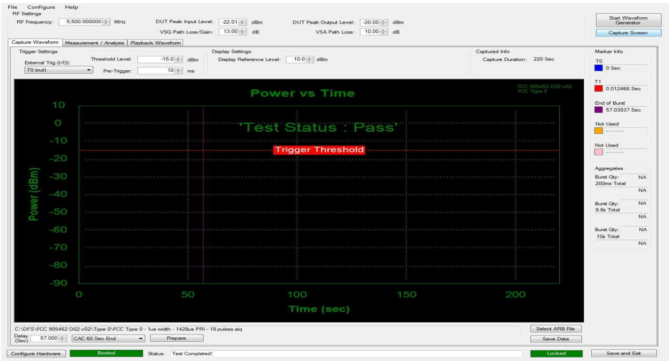
Figure 8.9-1: Radar burst at the end of the CAC
