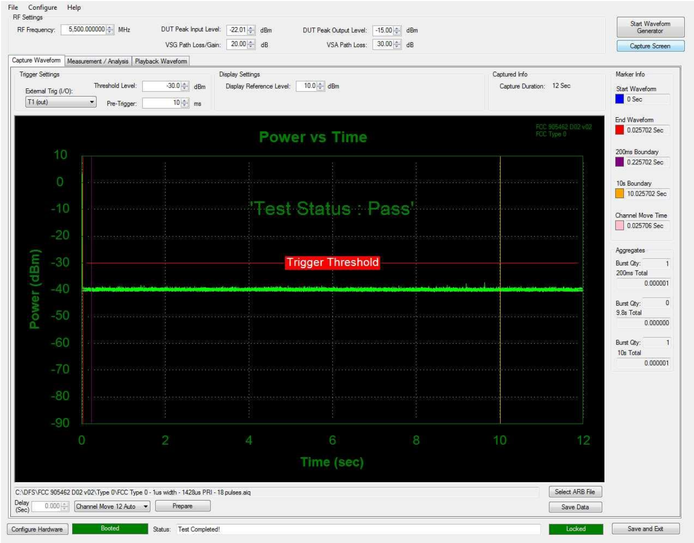
Figure 8.6-1: Channel closing transmission and move time
