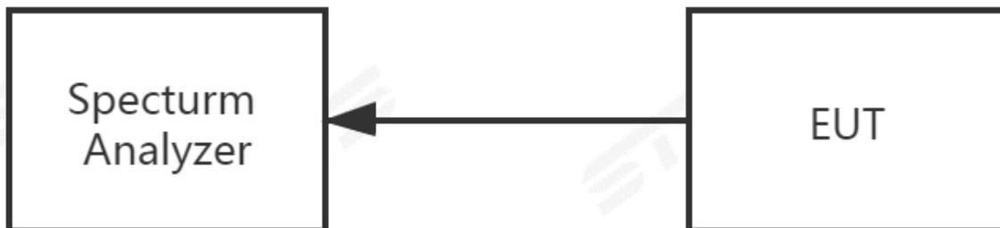
The EUT is connected to the Spectrum Analyzer; the RF load attached to the EUT antenna terminal is 50Ohm; the path loss as the factor is calibrated to correct the reading.
