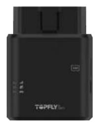
The tracker is using GNSS & LTE technologies and could collect device coordinates then transfer them via LTE network to the server. It provides customer with cost-effective, efficient and safety management. It has been widely used in commercial transportation, company vehicle fleet management, intelligent transportation, logistics, car rental, engineering machinery, marine transportation and other segments.
