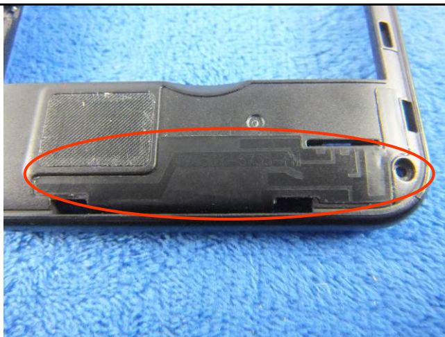
GSM/PCS/UMTS-FDD Antenna View
