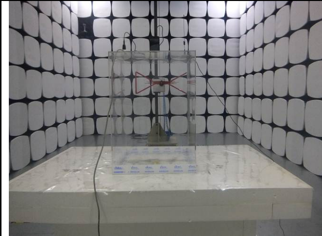
Radiated Spurious Emissions Test Setup Below 1GHz
