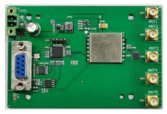
EC-RF650-C-ZM is a five channel fixed ultra-high frequency RFID reader and writer launched by EC-LINK company. It meets the ISO 18000-6C standard and operates at frequencies ranging from 840MHz to 960MHz. It has a compact appearance and outstanding read and write performance, supporting RS232 and RS485 interface data communication.
