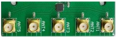
Note: The RF terminal is only connected to the antenna that needs to be used. Please do not open the software for unconnected antennas, otherwise empty space may damage the reader/writer!
