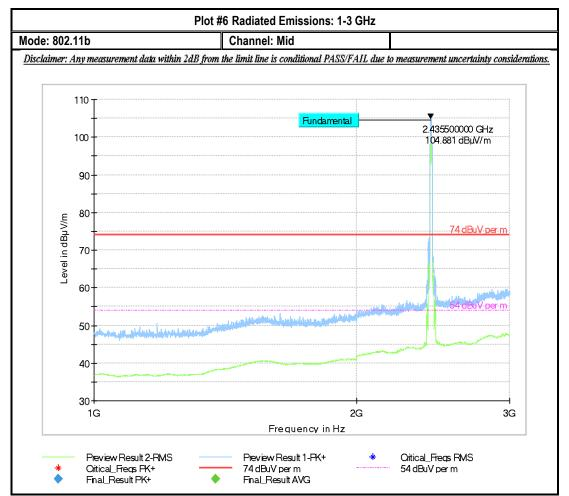
Note: The peak signal above is the transmit channel.
