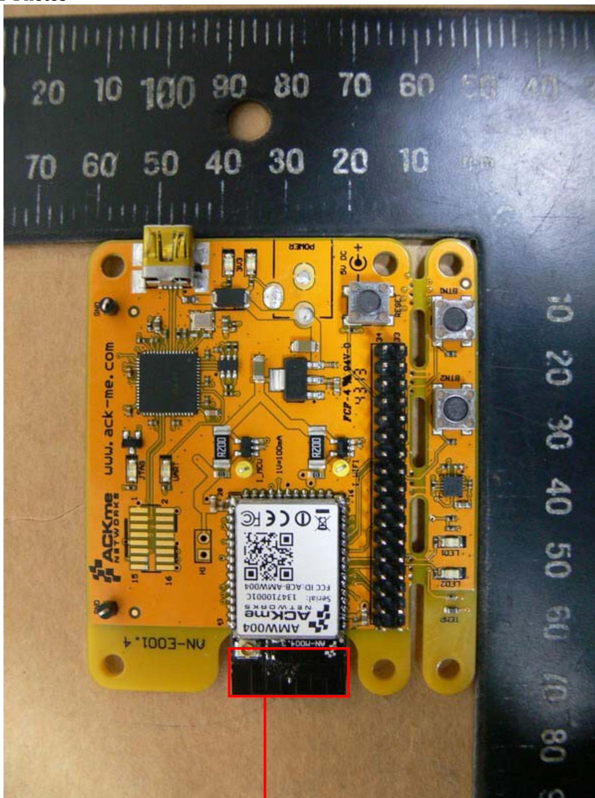
PCB antenna / 3.18 dBi
