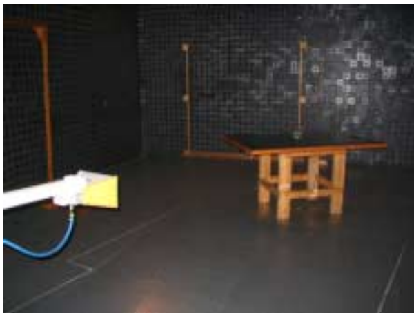
Photograph 9.2.2 Setup for radiated emission measurements, above 1 GHz
