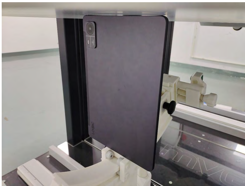
Body Left side (separation distance is 0mm)
