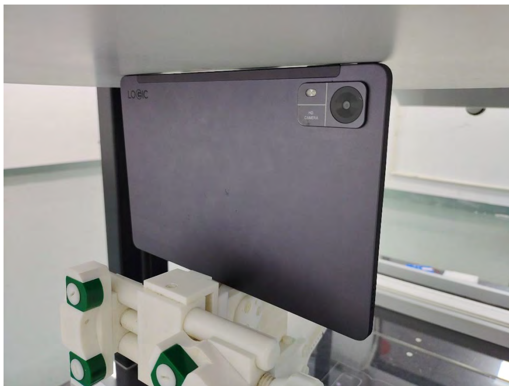
Body Top side (separation distance is 0mm)
