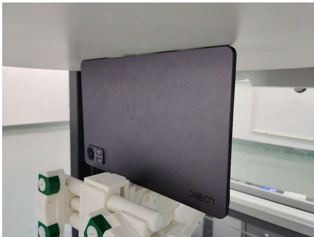
Body Top side (separation distance is 0mm)
