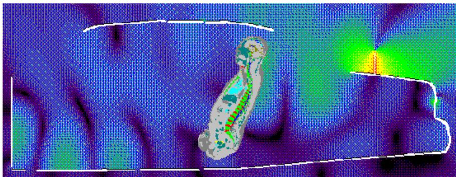
**Figure 1: Car passenger model exposed to a quarter wave antenna operating at 421.5 MHz
