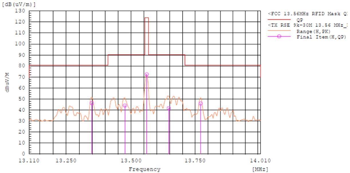
**Radiated E-Field Emission (Antenna Position 90°) : 13.110 – 14.010 MHz, Battery Discharging Mode**
