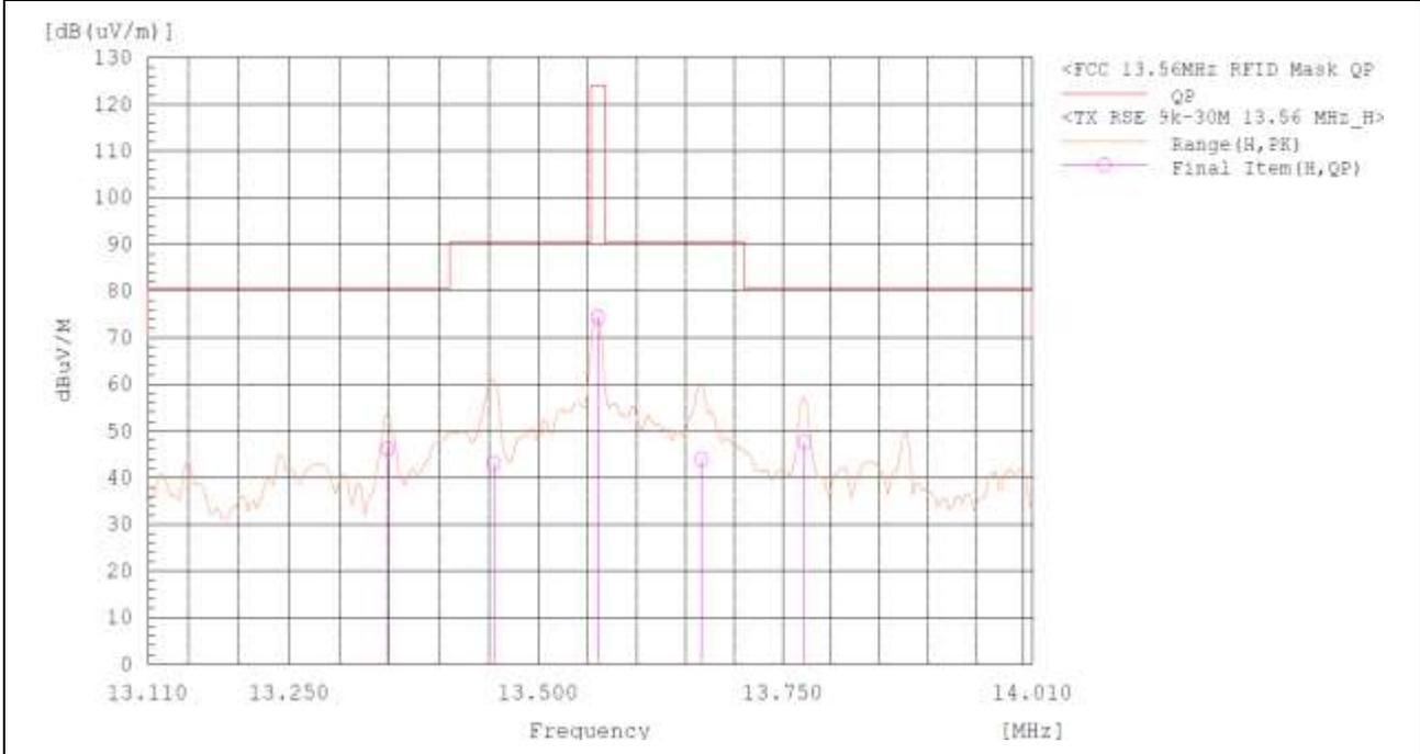
**Radiated E-Field Emission (Antenna Position 90°) : 13.110 – 14.010 MHz, Charging Mode**
