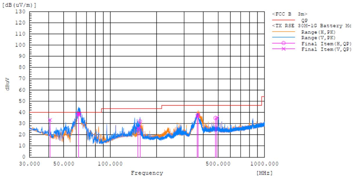
Test Mode Battery Discharging Mode
