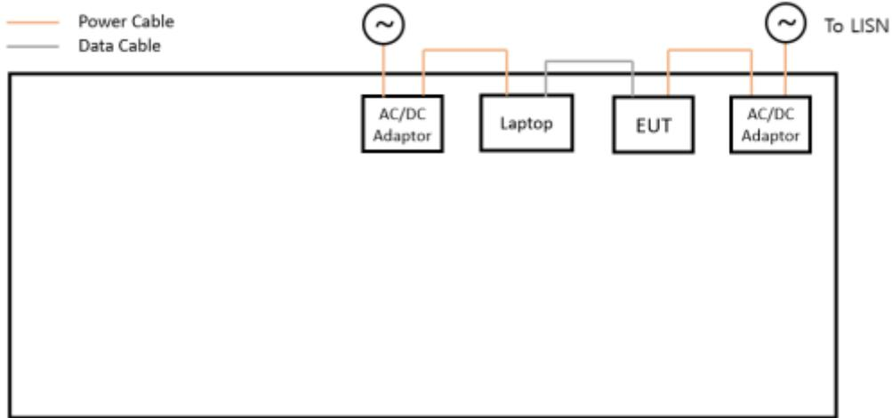
**Conducted Emission : Battery Discharging Mode**
