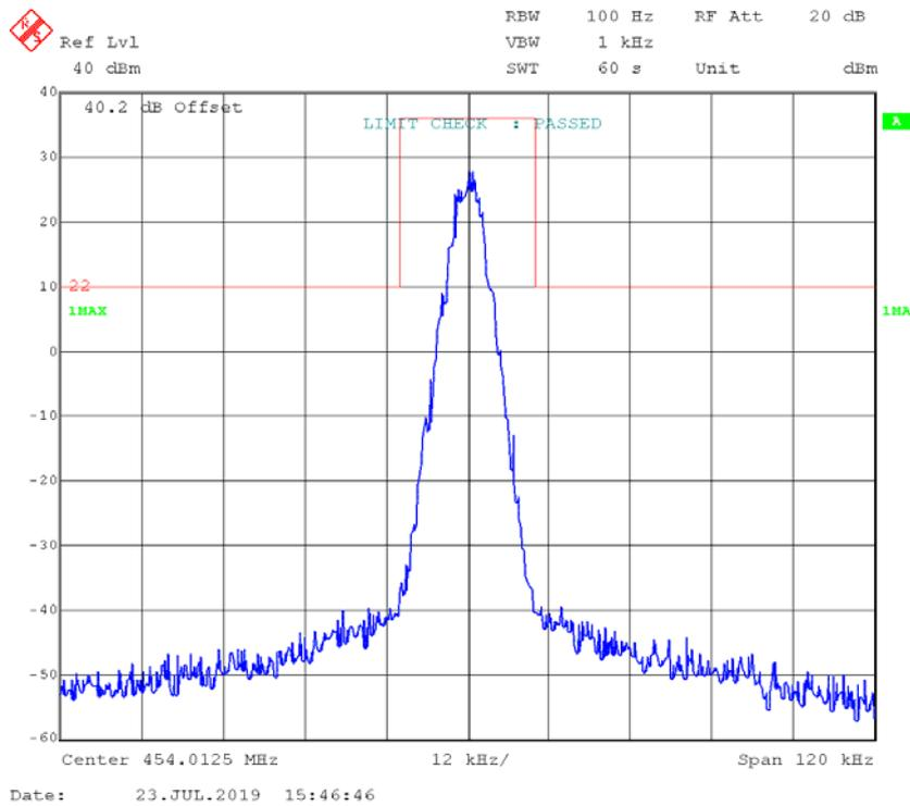
**4FSK,12.5 kHz, Low Power - Frequency 454.0125 MHz:**
