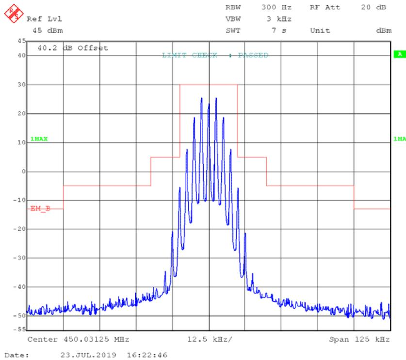
**4FSK,12.5 kHz, Low Power - Frequency 450.03125 MHz:**
