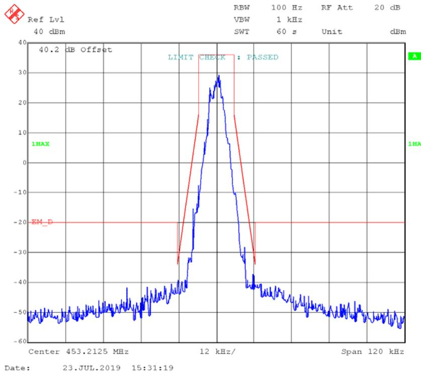
**4FSK,12.5kHz, Low Power - Frequency 453.2125 MHz:**
