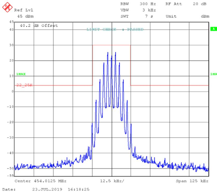
**4FSK,12.5 kHz, High Power - Frequency 454.0125 MHz:**
