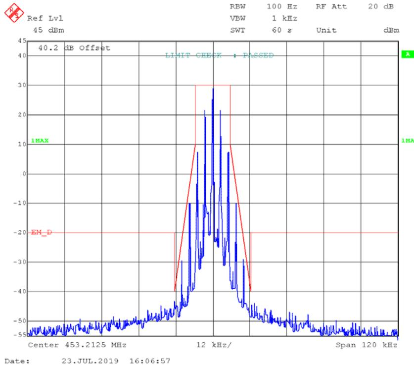
**4FSK,12.5kHz, High Power - Frequency 453.2125 MHz:**
