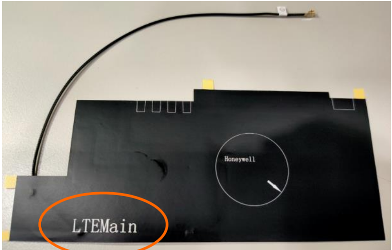
Antenna LTE Main _ No.3
