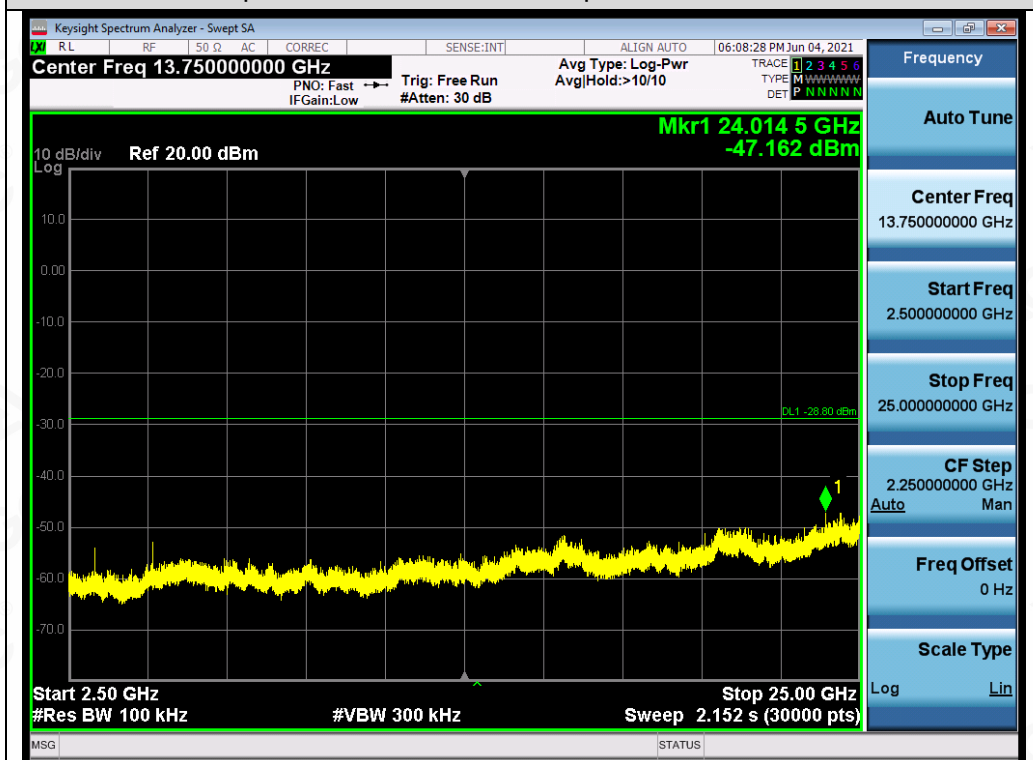
Test_Graph_EDR_ANT1_2441_2Mbps_Higher Band Emissions
