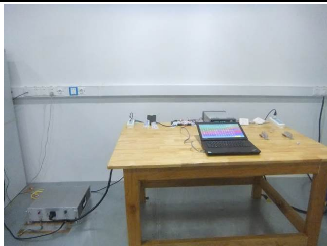
Conducted Emissions Test Setup – Front View
