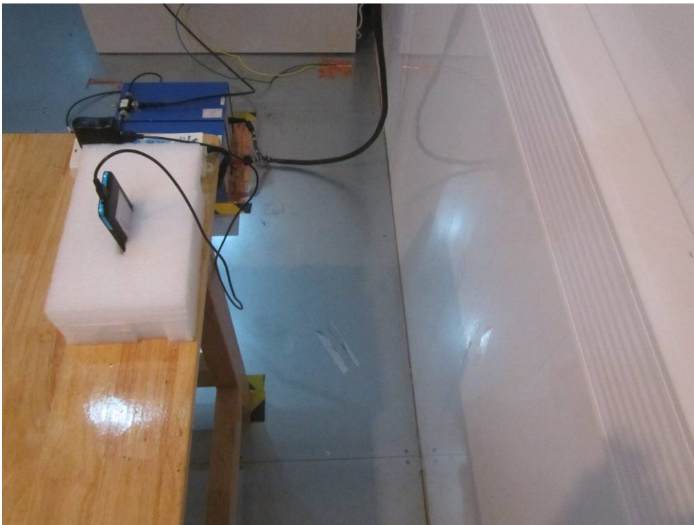
Conducted Emissions Test Setup Side View
