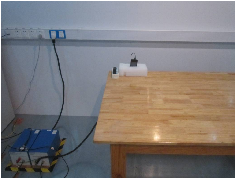
Conducted Emissions Test Setup Front View
