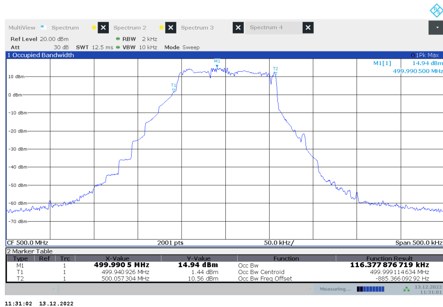
Plot 2: 500.000 MHz, max hold with frequency variation from 50 Hz to 15 kHz
