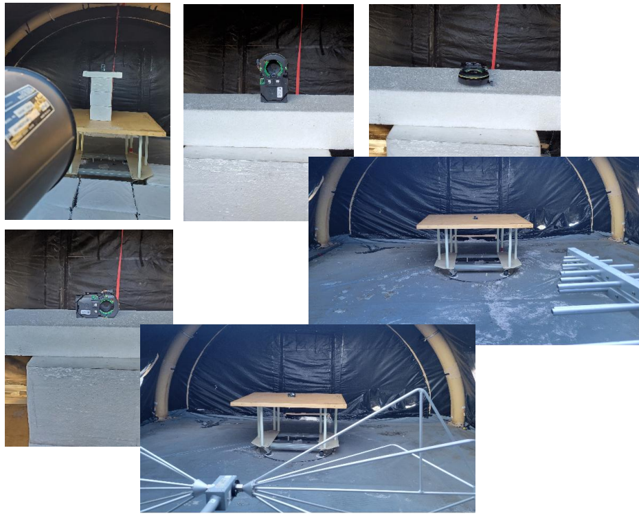
Figure 4: Radiated Emissions Test Setup Photograph(s).
