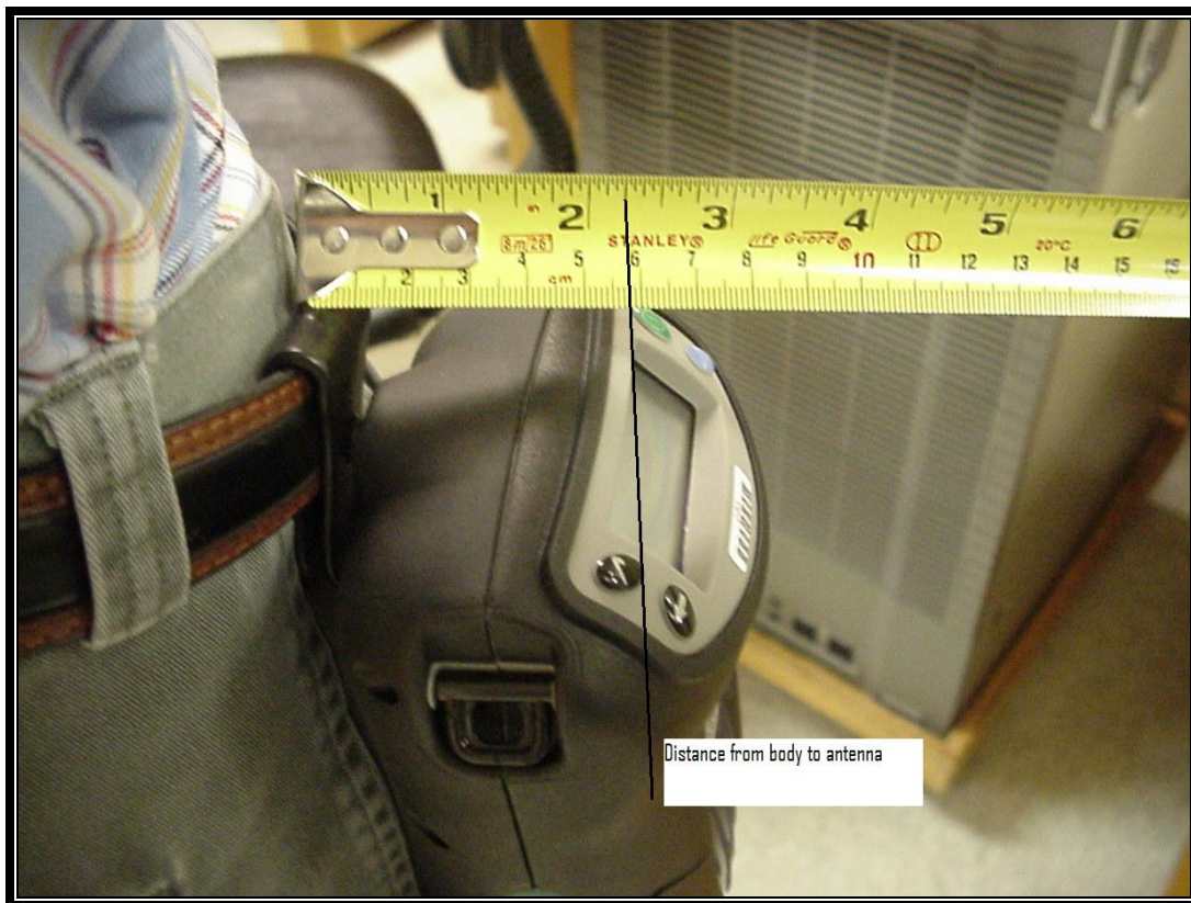
Photograph 9: Separation Distance Between CQ17718-G1 Antenna and Body
