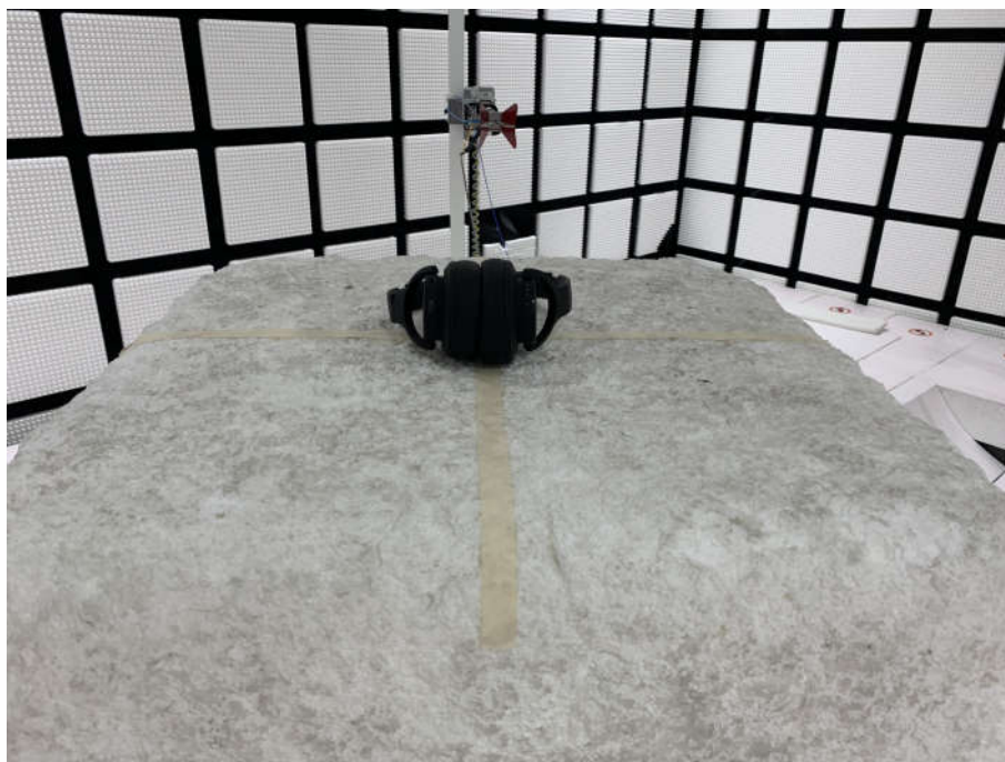
Radiated spurious emission Test Setup-2(Above 1GHz)
