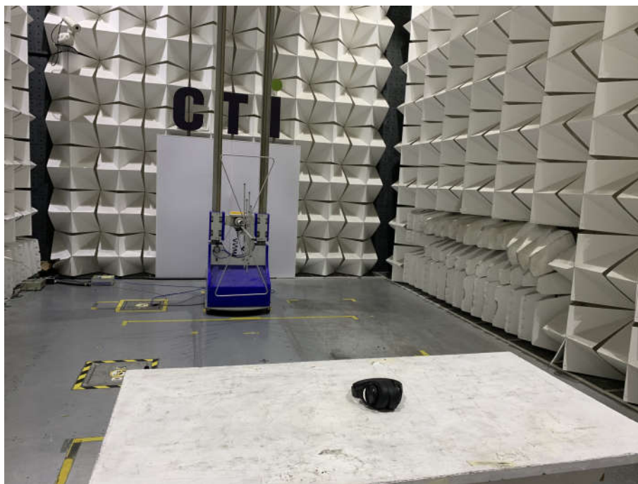
Radiated spurious emission Test Setup-1(Below 1GHz)
