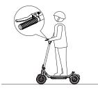
6 Press the brake lever to brake, and gently press the rear fender to assist the brake.
