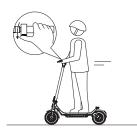
4 Press the THROTTLE button slightly on your right hand to start and rotate the handle to turn
