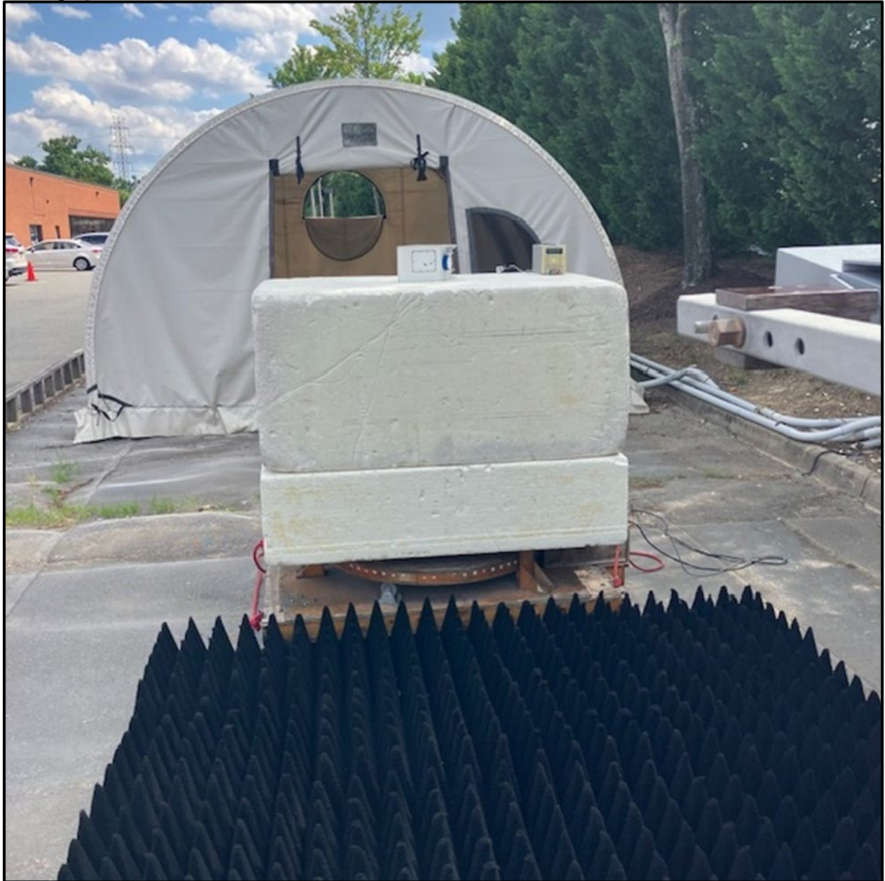
Photograph 2: Radiated Emissions Above 1 GHz – Front View
