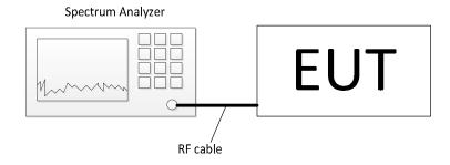
The relating measurements were carried out in a conducting manner. Therefore, the antenna connector was directly connected to a spectrum analyzer. The measurement procedure refers to part 11.11.2 and 11.11.3 of document [1].
