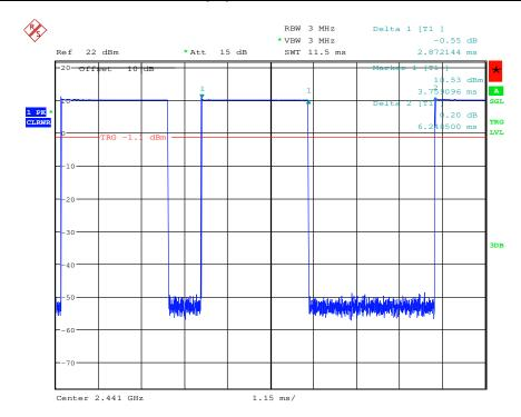
The signal combination was repeated after a short and a long Tx Cycle. Therefore the duty cycle could only be evaluated correctly, by looking at two consecutive TX periods.
