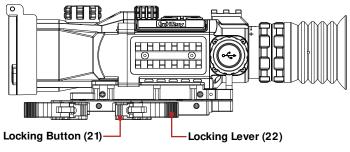
3. Press the levers closed to lock the mount in place. You will hear the lever and locking button click.
