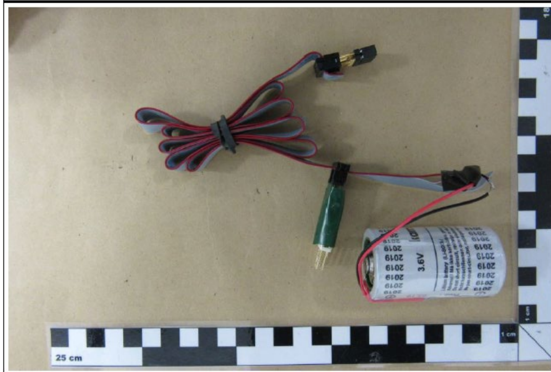
extension cable for modular approval test of module alone
