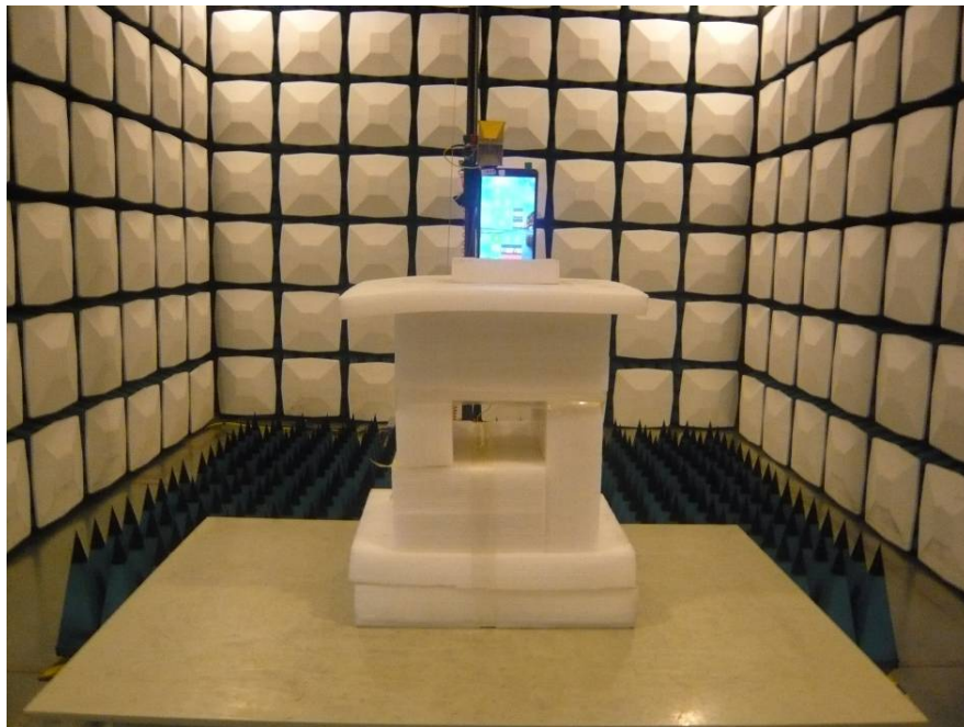
Radiated Emission View (Above 1GHz)
