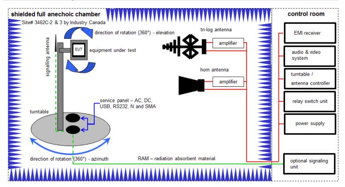
Measurement distance: tri-log antenna and horn antenna 3 meter
