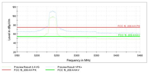
The variation of the peak and average amplitude @ 5.350 GHz is caused by an increased internal attenuation of the measuring receiver to prevent the equipment from overloading.
