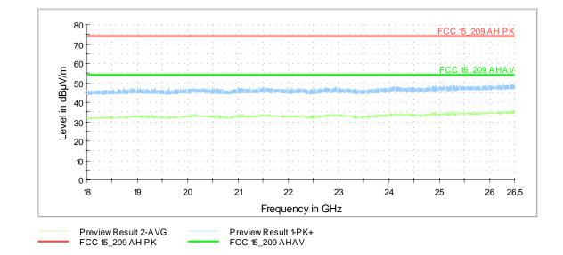
Operation mode 4: Spurious emissions from 18 – 26.5 GHz: (Preliminary plot)
