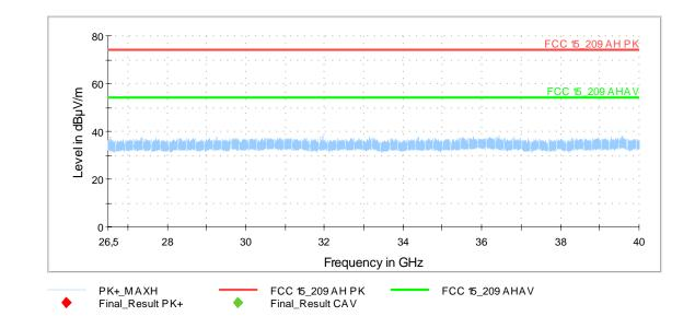
Operation mode 2: Spurious emissions from 26.5 - 40 GHz: (Preliminary plot)
