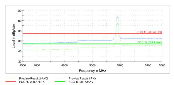
The variation of the peak and average amplitude @ 4.950 GHz is caused by the measuring system (preselect or); the variation @ 5.150 GHz is caused by an increased internal attenuation of the measuring receiver to prevent the equipment from overloading.
