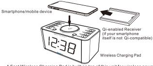
A Fast Wireless Charging Pad is built on top of this unit for wireless power transfer to any Qi-compatible smartphones or Qi-enabled receivers over a vertical distance of not more than 0.2 inches (5 mm)
