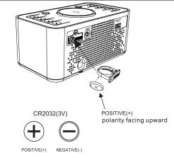
The lithium backup battery needs replacement when the LOW BATTERY indicator flashes, otherwise, the time and alarm settings will be lost/reset after a power outage
