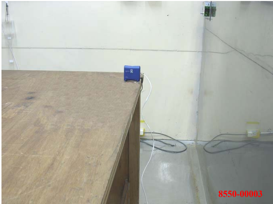
Photo 2: Conducted Emission Test Set-up
