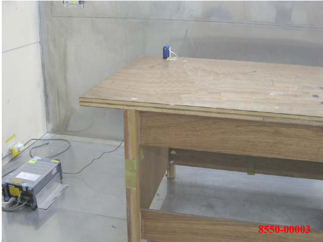
Photo 1: Conducted Emission Test Set-up
