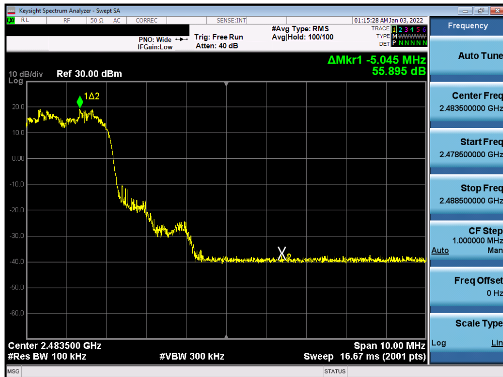
Plot 7-20. Band Edge Plot Antenna 3A (Bluetooth with Hopping Enabled, 8DPSK, ePA)
