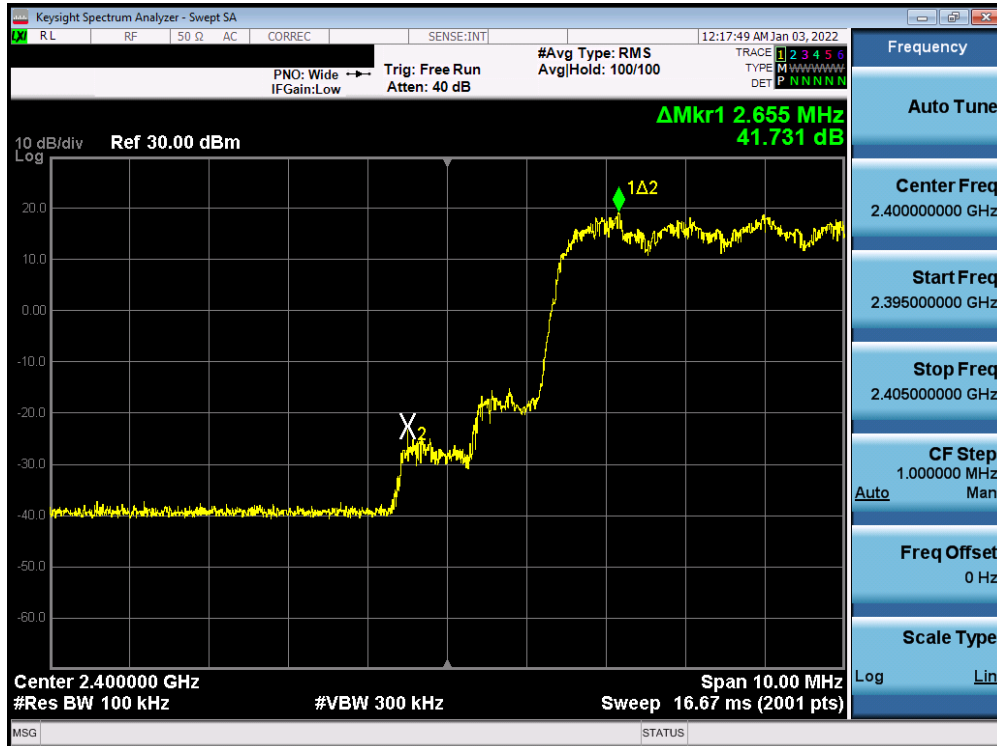
Plot 7-27. Band Edge Plot Antenna 1A (Bluetooth with Hopping Enabled, 8DPSK, ePA)
