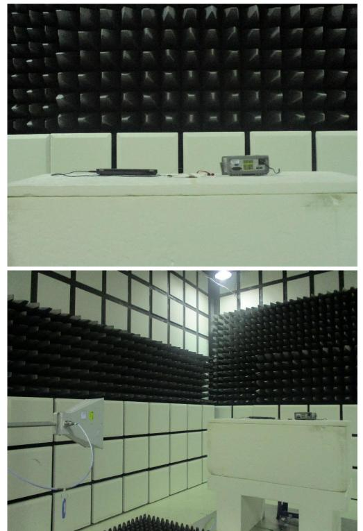
Radiated Emission Set up Photos (ABR-ANT-DF01)
