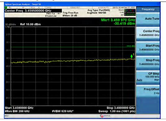
+3 dB above Out-of-band (single test signal) / 3.45 GHz Service(Ant1) / Downlink / 5G NR 80 MHz / Middle / Upper
