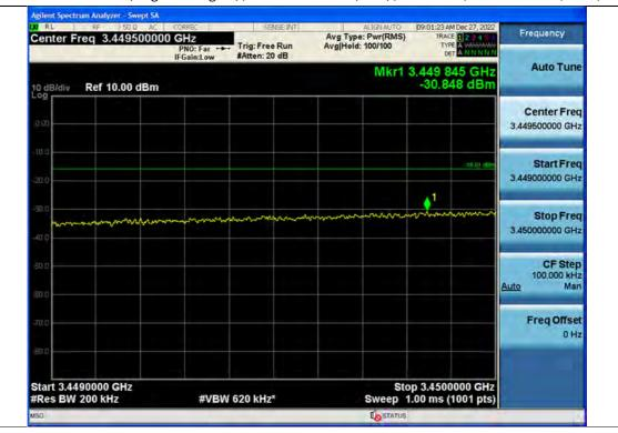
+3 dB above Out-of-band (single test signal) / 3.45 GHz Service(Ant1) / Downlink / 5G NR 60 MHz / Low / Lower
