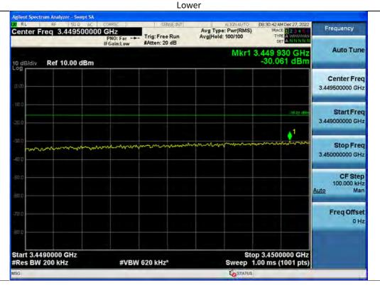
+3 dB above Out-of-band (single test signal) / 3.45 GHz Service(Ant1) / Downlink / 5G NR 100 MHz / Middle / Upper
