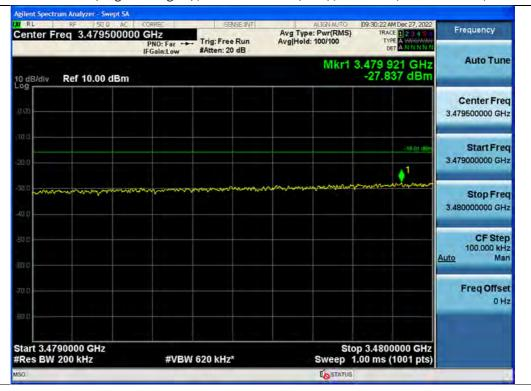
+3 dB above Out-of-band (single test signal) / 3.45 GHz Service(Ant1) / Downlink / 5G NR 40 MHz / Middle / Upper
