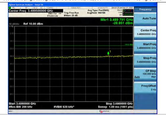
Out-of-band (single test signal) / 3.45 GHz Service(Ant2) / Downlink / 5G NR 60 MHz / High / Lower
