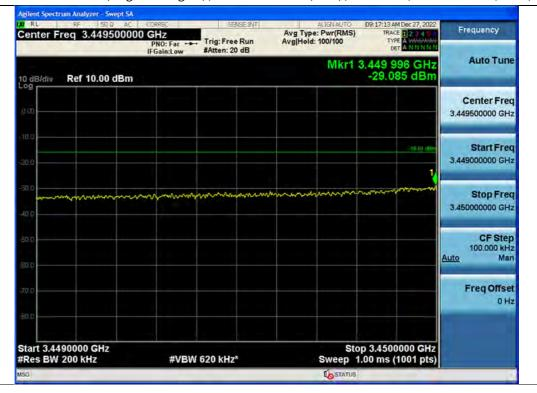
+3 dB above Out-of-band (single test signal) / 3.45 GHz Service(Ant2) / Downlink / 5G NR 40 MHz / Low / Upper
