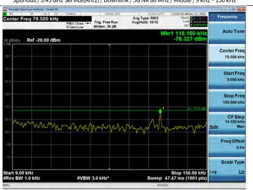
Spurious / 3.45 GHz Service(Ant1) / Downlink / 5G NR 80 MHz / Middle / 9 kHz ~ 150 kHz
