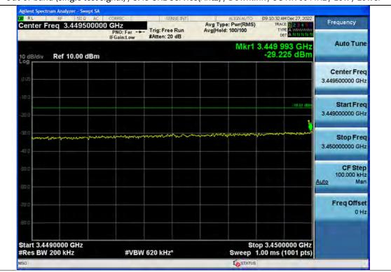
Out-of-band (single test signal) / 3.45 GHz Service(Ant2) / Downlink / 5G NR 60 MHz / Low / Lower
