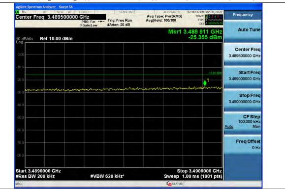
Out-of-band (single test signal) / 3.45 GHz Service(Ant2) / Downlink / 5G NR 20 MHz / Middle / Lower
