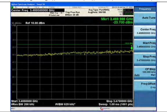
Out-of-band (single test signal) / 3.45 GHz Service(Ant1) / Downlink / 5G NR 60 MHz / Middle / Lower
