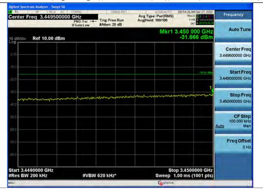
+3 dB above Out-of-band (single test signal) / 3.45 GHz Service(Ant1) / Downlink / 5G NR 80 MHz / Low / Upper
