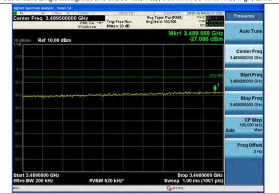
Out-of-band (single test signal) / 3.45 GHz Service(Ant1) / Downlink / 5G NR 60 MHz / High / Lower
