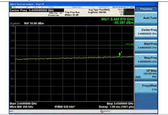
Out-of-band (single test signal) / 3.45 GHz Service(Ant1) / Downlink / 5G NR 100 MHz / Middle / Lower
