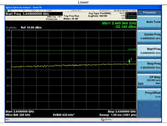
+3 dB above Out-of-band (single test signal) / 3.45 GHz Service(Ant2) / Downlink / 5G NR 100 MHz / Middle / Upper
