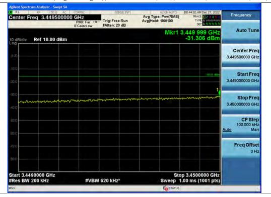
+3 dB above Out-of-band (single test signal) / 3.45 GHz Service(Ant2) / Downlink / 5G NR 80 MHz / Low / Upper
