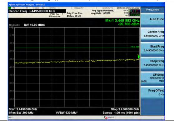
Out-of-band (single test signal) / 3.45 GHz Service(Ant1) / Downlink / 5G NR 80 MHz / Low / Lower
