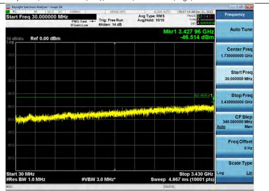
Spurious / 3.45 GHz Service(Ant2) / Downlink / 5G NR 80 MHz / High / 30 MHz ~ 3 430 MHz
