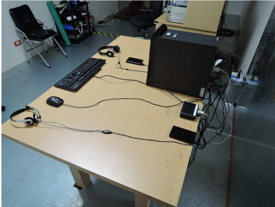
Photograph 5: Set-up for for Mains Conducted testing Back
