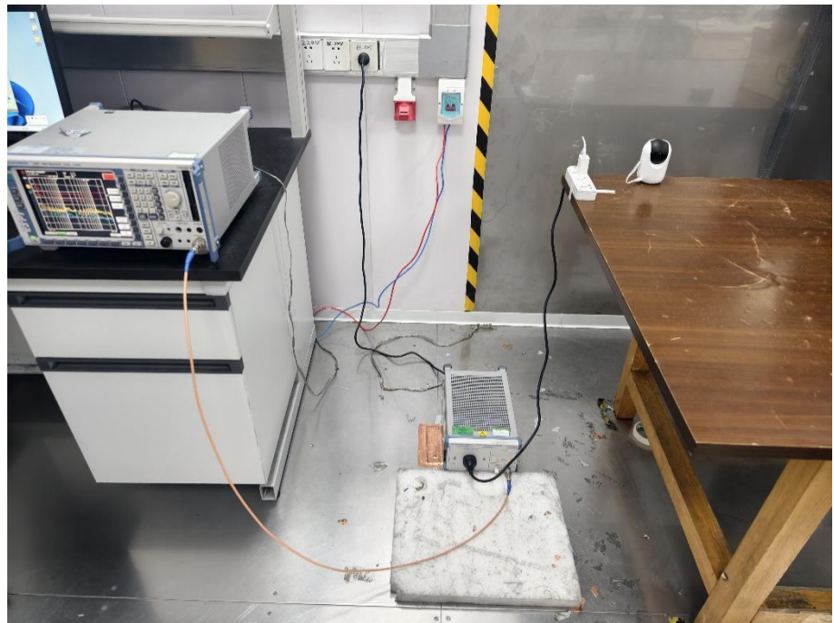
Conducted Emission Test Setup
