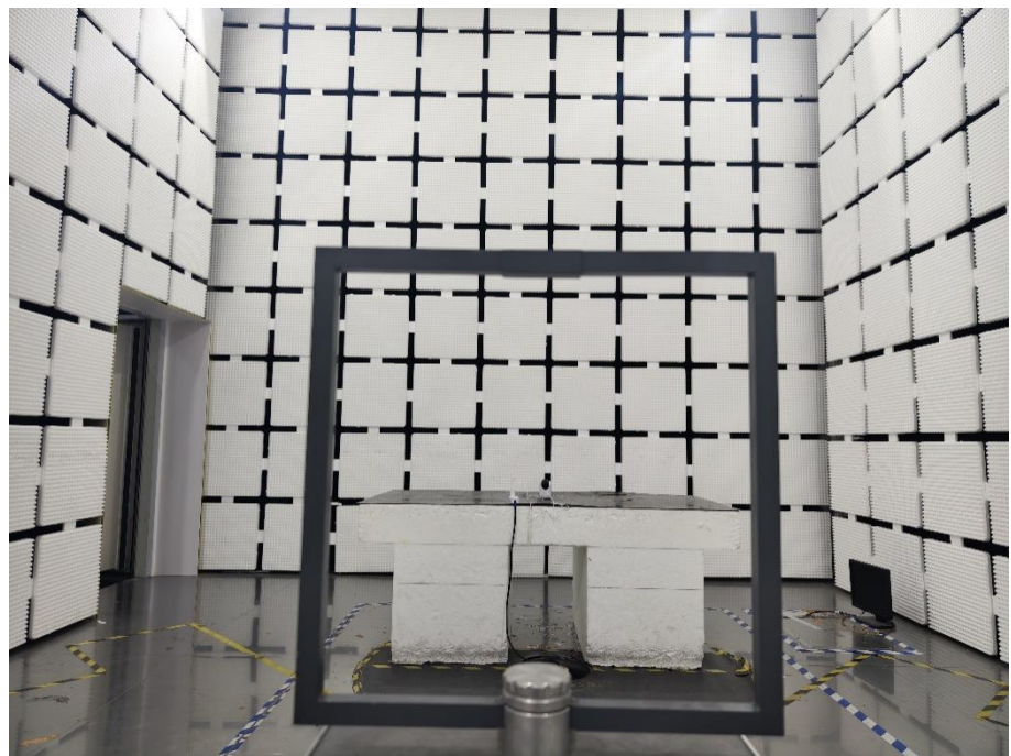
Radiation Emission Test Setup (Below 30MHz)
