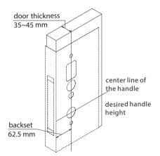
Note 1: Align the template along the vertical center line of the mortise (H) at the desired handle height, and tape it to door.
