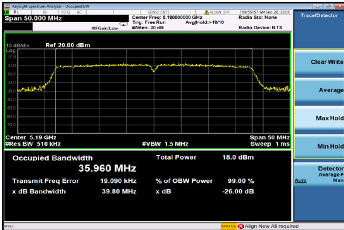
**26dB / 99% Band Width Test Data CH-Mid**
