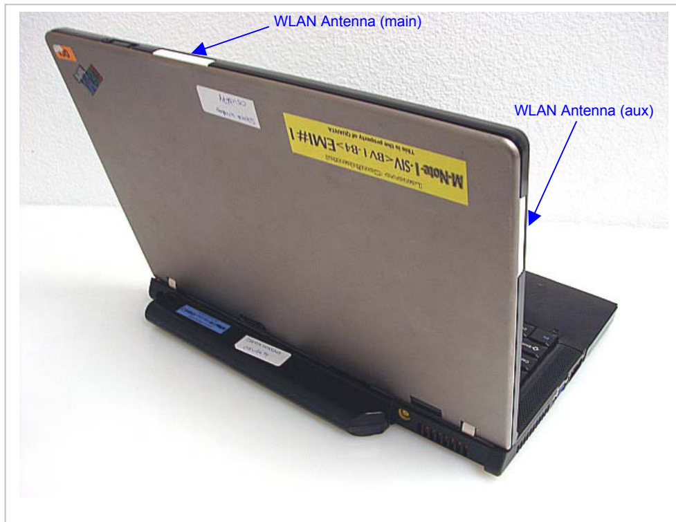
Rear View Levono M-note – Metal LCD Cover
